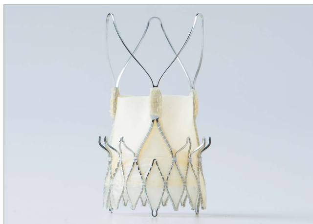
Figure 1. The ACURATE neo prosthesis. Stabilisation arches allow axial self-alignment of the prosthesis, the upper crown allows supra-annular anchoring and the lower crown is designed for minimal protrusion in the left ventricular outflow tract. The skirt acts against paravalvular leakage.
