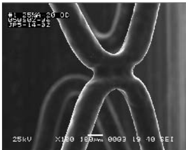
Figure 2. A deployed Endeavor Resolute stent after tracking 3 times in a 5 Fr guide catheter.
