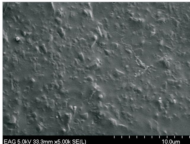
**Figure 1.** MiStent SES utilises crystalline sirolimus in a polymer coating (scanning electron microscopy).
