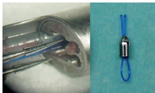
Figure 2. LEFT. Window of therapeutic catheter with vacuum port and needles. RIGHT. Suture clip.
