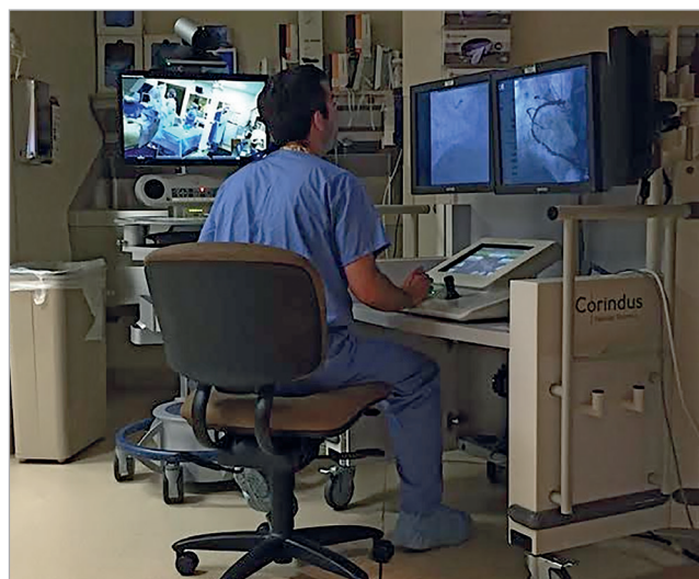
Figure 1. Performance of PCI by a physician operator outside the confines of the procedure room housing the patient. The operator is seated within the robotic cockpit located in an isolated room. Two monitors display real-time fluoroscopy and cineangiography images. A third monitor displays real-time haemodynamic and electrocardiographic data. To the left of the operator is a telecommunications device providing real-time video and audio connectivity to the procedure room housing the patient. PCI: percutaneous coronary intervention
