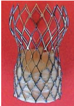
Figure 2. The CoreValve stented valve consists of a self-expandable nitinol stent in which a trileaflet valve is mounted. The nitinol frame has a diamond cell design with different strut lengths and widths to accommodate expansion to a non-uniform cylindrical shape. The lower or most distal part has a high radial force to push aside the native aortic leaflets and preventing recoil. The middle part is constrained to avoid interference with flow through the coronary ostia and hosts the tissue valve. The upper or proximal part implants itself on the ascending aorta, assuring anchoring and alignment of the implant. The valve is made of single layer of porcine pericardium constructed in a trileaflet configuration, which are attached to a scalloped skirt (also made of a single layer of porcine pericardium) using PTFE sutures. The valve is sutured to the nitinol frame with 5.0 PTFE sutures. The stented valve is crimped onto a 21.0 Fr delivery catheter covered by a protective sheath holding the prosthesis in a collapsed position.
