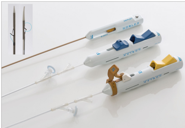
Figure 1. Description of the NobleStitch EL system. The NobleStitch EL suture delivery system consists of two dedicated catheters (NobleStitch S and NobleStitch P) to capture and suture the septum secundum and the septum primum using a 4-0 polypropylene suture. The distal end of each NobleStitch suture delivery has a suture-carrying arm which opens inside the heart to engage the septum secundum and primum and an internal needle which pierces through the septum tissue picking the suture up in the opened carrying arm. A third element, the KwiKnot catheter, is advanced over the septum secundum and septum primum sutures to secure the stitch and trim the excess suture material.
