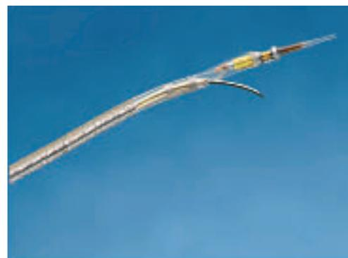
*Fig. 1: Pioneer crossing device TransAccess double lumen catheter with puncture needle and integrated phased array 20 MHz IVUS transducer.*
