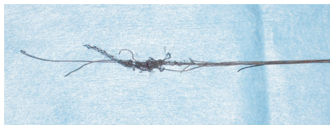
Figure 9. Picture of the retrieved fractured wire, stent and multiple wrapped wires with balloon.
