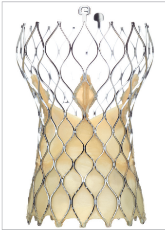
Figure 1. The CoreValve Evolut R. The CoreValve Evolut R has been redesigned to provide more consistent radial force across the sizing range with modified cell geometry to improve conformability to the aortic annulus. The new valve release mechanism has a paddle design to prevent hang-ups and the porcine pericardial leaflets are treated with alpha-amino oleic acid (AOA®) to retard mineralisation.
