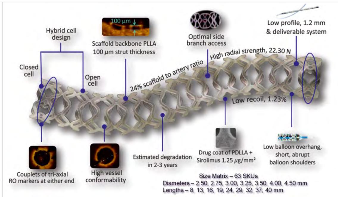
Figure 1. Design of the MeRes100 bioresorbable vascular scaffold stent platform.
