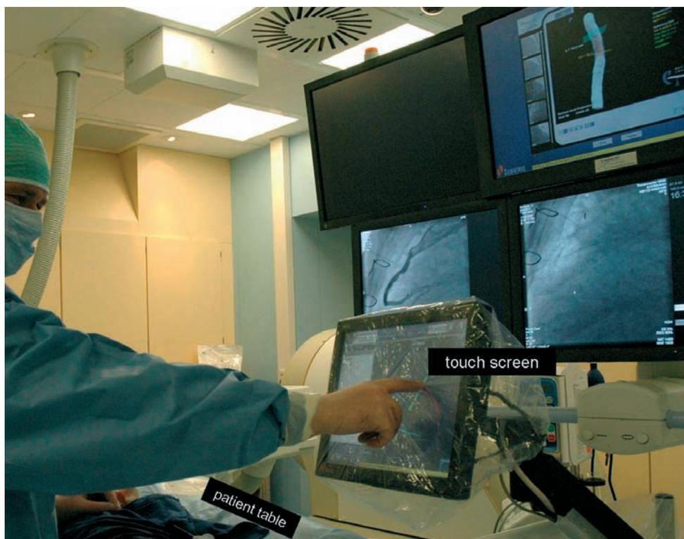
Figure 3. How does the physician operate the magnetic navigation? In the current system incorporated with 3 dimensional (3D) vessel image, the physician can align the direction of the guidewire by touching the 3D coronary path on the screen located beside the patient table. Alignment of the wire direction and advancement of the wire can be performed by one physician. The wire direction is systematically changed prior to advancement.
