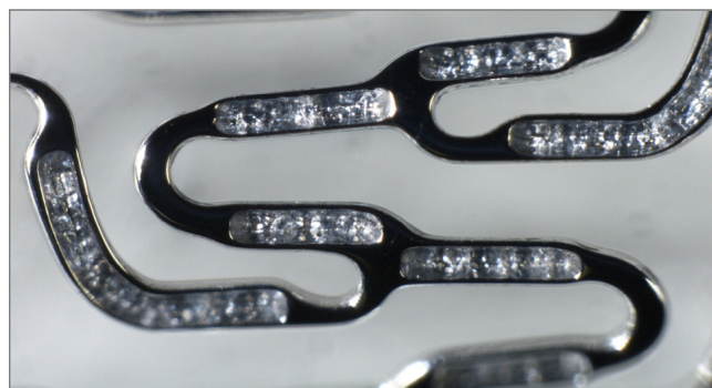
Figure 1. Macro picture of the Cre8 stent. The stent structure with the abluminal reservoirs filled-in with Amphilimus formulation is visible.
