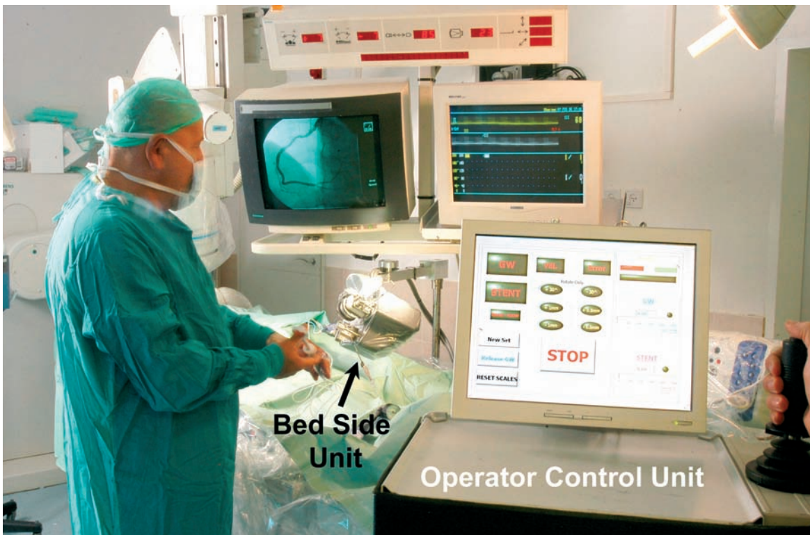
Figure 3. The set-up of the prototype system in the catheterization laboratory. The console was operated from inside the catheterization room. The bed-side unit was attached to the catheterization bed by an adjustable arm. An operator was present at the table for contrast injections and balloon dilatations.
