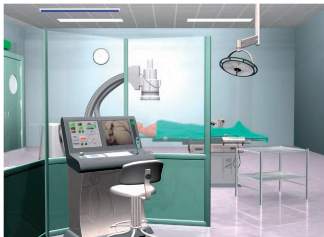
Figure 1. A prospective overview of the cath lab set-up for the remote navigation system. A bed side unit attached to the patient bed is controlled by the console in an X-ray protected environment, either within the catheterization room or at another location. All the procedural operations can be controlled from the console, including wire and device manipulations, balloon inflations, coronary injections and table and C-arm orders.
