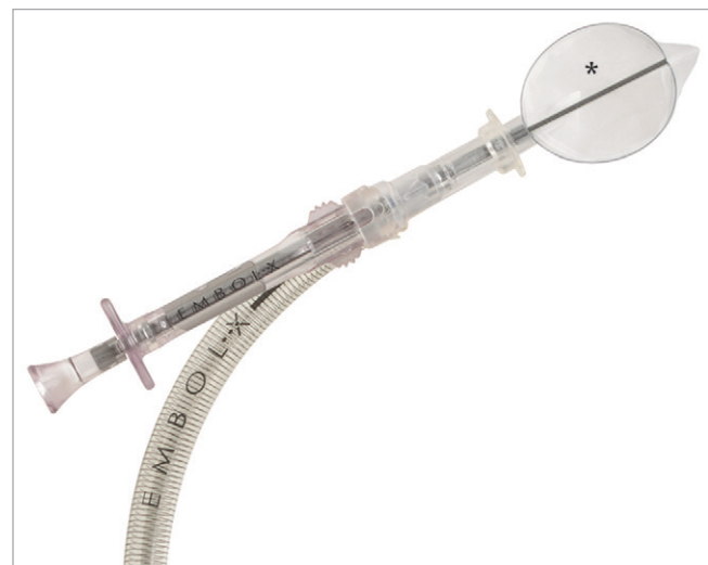
Figure 5. The Embol-X device is introduced via a sidearm of a modified 24 Fr intra-aortic cannula. The polyester mesh (*) captures debris with a diameter >120 µm.
