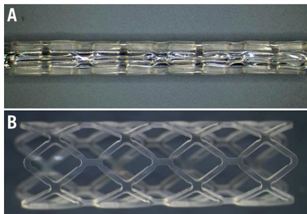
**Figure 1.** PLA stent. Illustration of PLA stent with a Palmaz-type design (200  $\mu\text{m}$  thick and 15 mm long) processed from moulded tubes by laser cutting crimped on a balloon catheter (A), and after deployment (B).
